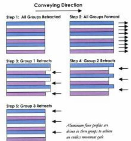
The TNS floor from Spiro takes this technology several steps further. First of all, it only uses two groups of planks rather than three, but also of importance, is that the planks overlap, preventing leakage of material occurring beneath the floor.
