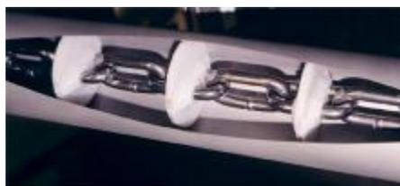
*Cutaway of Tube Chain Conveyor*
