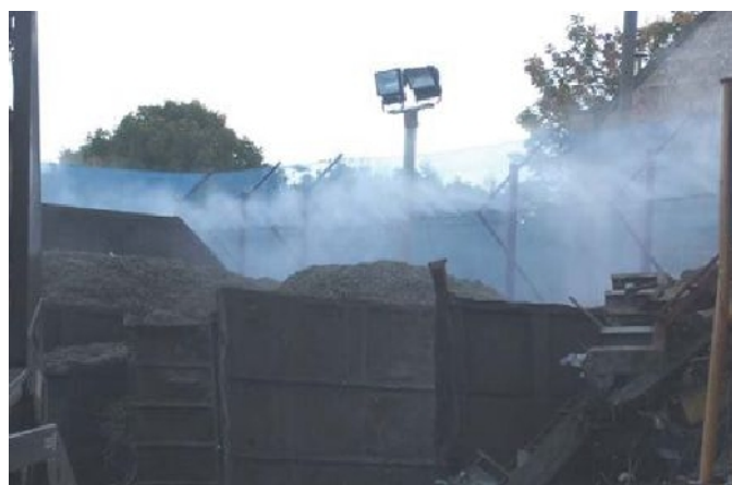
Perimeter fog around a metals recycler yard
