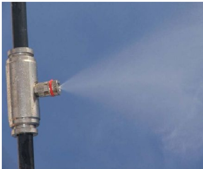
Pressurised water fogging nozzle
