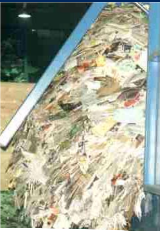
Typical Spiro Conveyor Floor Storage bunker with hydraulic activated doors.
